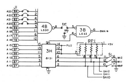
Figure 2-1. Memory Address Detection
