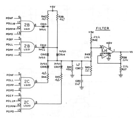
Figure 2-14. Phase Detector and Filter
