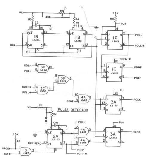
Figure 2-15. VCO and Timing Generator
