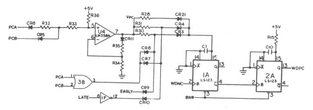
Figure 2-13. Write Precompensation Circuit
