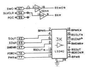
Figure 2-3. Control Signal Buffers
