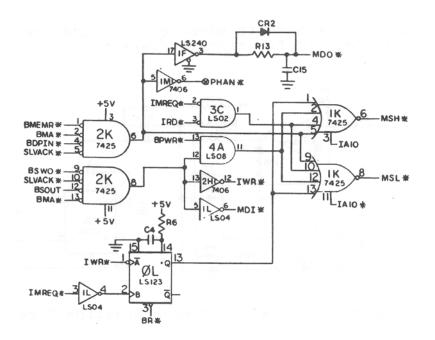
Figure 2-12. Memory Control Circuit
