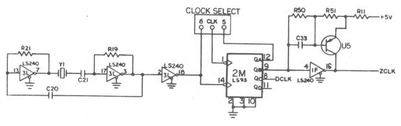
Figure 2-6. Clock Circuit
