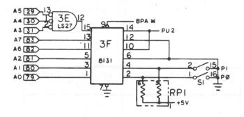
Figure 2-2. Port Address Detection
